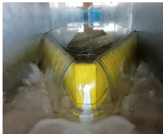
Fig. 3 Duckbill spillway with an 8-cm nose and an effective length of 1.8 meters.
